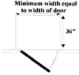
All landings are to be sloped a maximum of 1/4" per foot to drain water.
