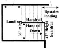
Private stairways and landings are required to be a minimum of 36" in width. Handrails are required on one side of an interior stairway and continuous between landings. Stairways with less than 4 risers are not required to have handrails.
