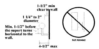
The handgrip portion of handrails shall be round and not less than 1-1/4" or more than 2" in cross-sectional dimension. If not round then the handgrip portion must have a 2-1/4" maximum cross section and a perimeter of 4" minimum to 6,25" maximum,
