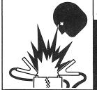
Equipped with 12/24 volt start system. Do not jump start. See Operator's Manual.
