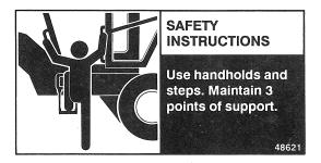
This safety sign is located on both sides of the cab.
