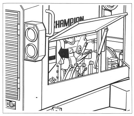
This safety sign is located on both sides of the fan shroud. On some models it is located on the frame.
