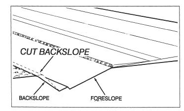
If the backslope is insufficient or if you are building a new road make a pass to cut the backslope. See this section -Right-hand 'V' Ditching page 10-22.
