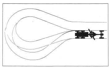
Upon completing the turn, turn the wheels right and articulate the frame straight.
