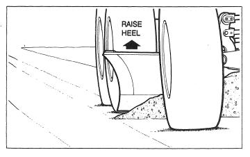
As you make a final pass at the edge of the shoulder, raise the heel of the moldboard to feather the material and use the tandem wheels to compact any remaining material.
