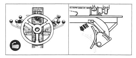
If using an articulated grader, ensure the articulation lock pins are removed before articulating, and install them when not using the articulation function. For right-hand leveling articulate the frame to the right. If the drive wheels lose traction, then reduce the articulation angle. This will decrease the cutting angle and side thrust allowing the drive wheels to regain traction. Deposit the windrow between the tandem wheels. Spread the windrow over the new surface until it is smooth.
