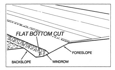
Reposition the moldboard to make a cleanup pass to spread the windrow created by the flat bottom cut up onto the shoulder. Spread this material and finish the final grade.
