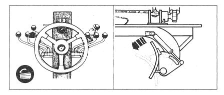
If using an articulated grader, ensure the articulation lock pins are removed before articulating, and install them when not using the articulation function. For left-hand leveling articulate the frame to the left. If the drive wheels lose traction, then reduce the articulation angle. This will decrease the cutting angle and side thrust allowing the drive wheels to regain traction. Deposit the windrow between the tandem wheels. Spread the windrow over the new surface until it is smooth.
